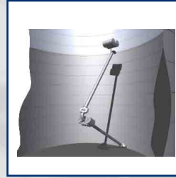
Floating Suction Lines
